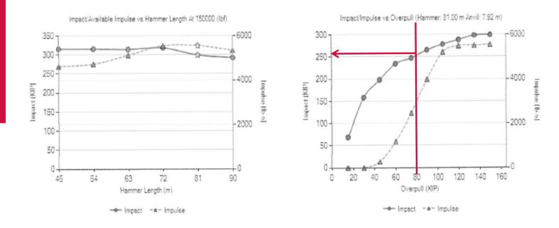
With a calculated impact of 260Klbs they stayed quite safely away from the tensile limit of the 2-3/8" Regular Box (375Klbs) or even 80% of the tensile yield (300Klbs).
